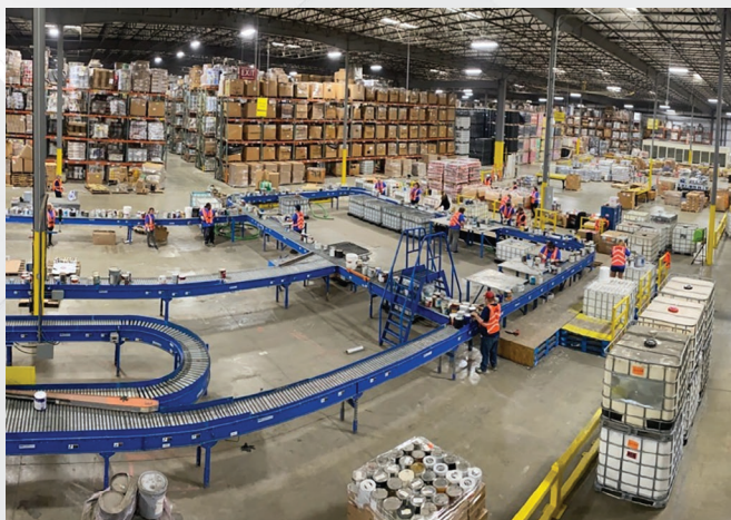
GDB's conveyor system at its Nashville HQ for inbound paint segregation prior to recycling.
